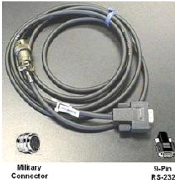
Figure 1-20 RS-232 local communication cable
