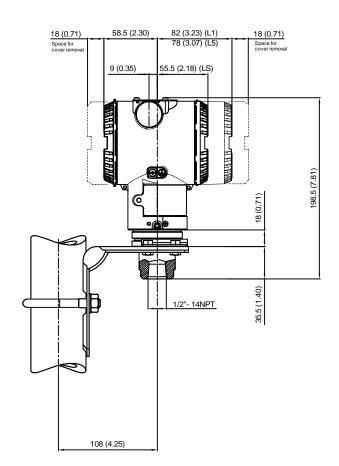
Vertical or horizontal Ø60mm (2.36in.) pipe mounting
