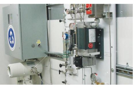
The NGC8203 gas chromatograph has a special column set to analyze the components found in low Btu "Landfill" gas.
