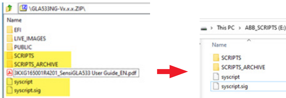
Figure 45 Extracting files to the USB storage device
