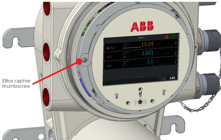
Figure 14 Unscrewing the EBox Captive Thumbscrew
