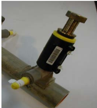
ELECTROFUSION OF KEROTEST REPAIR KIT TO ALDYL-A TEE
