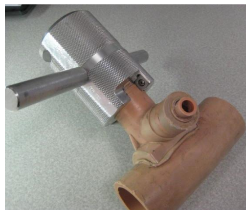
Removes material from the head of Aldyl-A Tapping Tee
