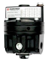
A pneumatic air volume booster reproduces a low flow control signal with a greater flow regulated output pressure. It uses an unregulated input pressure to maintain a regulated output pressure under flowing and non-flowing conditions.
