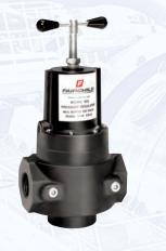
A pressure regulator reduces an unregulated high input pressure to a regulated lower output pressure. Its primary function is to maintain the regulated output pressure under flowing and non-flowing conditions.
