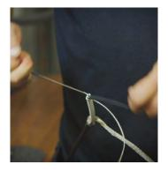
Expose inner wire and remove excess black sheathing.
