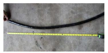
With the end of the heat trace bundle, measure from the sample point to the device (or 36" from end).
