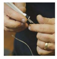
Once the wire is exposed, attache the patns (frog legs). Be sure to not lose any part of hte fiber wire; you will need to start over if fiber is missed.
