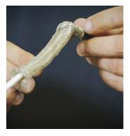
Collapse outer braided ground sheath. Compress and open a space between the braids. Remove the sheath from the wire by pulling the wire through the opening. Do not cut the wire.
