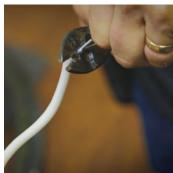
Insert each wire into a pin terminal. Crimp each terminal to secure.
