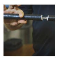
Bend and score to expose wires until outside wrap is completely separated.
