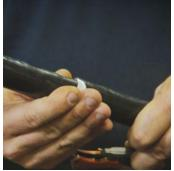
Score at mark. Do not cut through to the wires.
