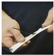
Measure to the Pants (or Frog Legs) about 8" from the end of the white wire sheath (or termination point).
