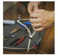
Once the wire is exposed, the tubes can be removed.
