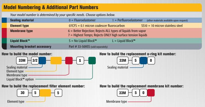
Replacement filter and membrane kits contain 5 each. O-ring replacement kit contains all assembly o-rings.
